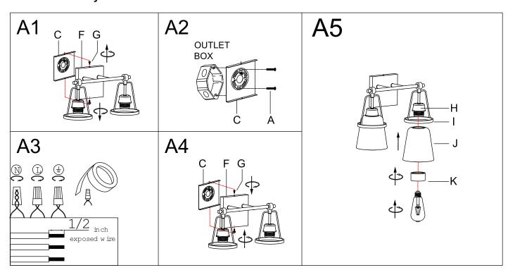
Step A1 » Unscrew studs (G) from back plate (F), then set them aside for later installation.
