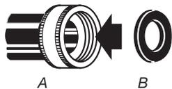
Washer must be connected to water faucets with new inlet hoses (A) with flat washers (B) (not provided). Do not use old hoses.
