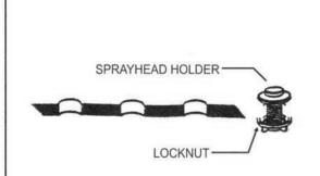
Separate locknut from sprayhead holder and insert sprayhead holder through sink. Reassemble and tighten locknut.
