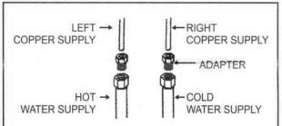
Carefully bend the copper supplies to meet the supply lines. Use the palms of your hands to bend, so as to avoid kinking.
