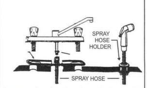
Insert spray hose from above through holder then up through center hole in sink and thread through plastic gasket. Attach spray hose to faucet fitting and tighten.
