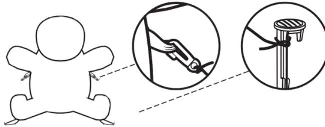
For inflatables under 9-feet tall, install at least three upper tie downs. For inflatables over 10-feet tall, you will need to install four or more upper tie downs, depending on the inflatable.
