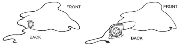
Lay your inflatable out on the ground. The fan will be on the back side of the inflatable. Ensure that the deflation zipper on the back of the inflatable is closed. Plug the fan into a Class A GFCI-protected receptacle to start inflating your inflatable.
