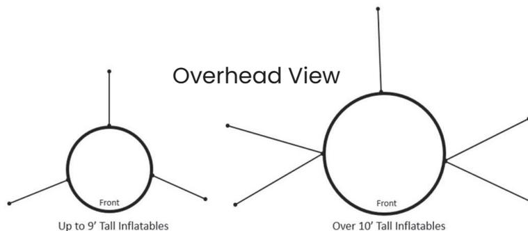
To properly secure your inflatable, install the upper tie downs according to the above graphic. Note that two of the side tie downs must angle forward by at least 30 degrees. Adjust stakes as needed to assure that the inflatable is fully upright and positioned correctly. When the inflatable is correctly positioned and all stakes have been placed, push all of the stakes fully into the ground.
