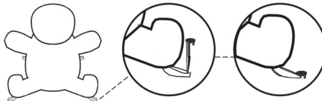
When fully inflated, locate all of the tie-down points around the base. Place a stake through the loop and press the stake about  $\frac{2}{3}$  of the way into the ground (you will insert these fully later). These stakes help hold the inflatable upright and prevent the wind from moving your inflatable.
