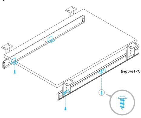
Screw the shelf through the slot on shelf tab from the bottom.
