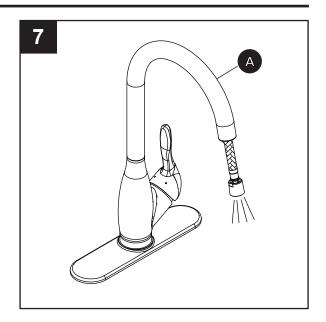
8. Re-assemble spray head. Push the button of the spray head to alternate the spray between stream and spray.
