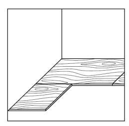
Note: plywood is a water-sensitive subfloor that may become damaged or
