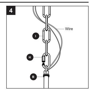
Feed the chain (I) and wire through the decorative nut (E) and the ceiling plate (G) and mounting bracket (C). Then use an open link (H) to connect the chain (I) to the chain loop (F) preassembled to the mounting bracket (C).
