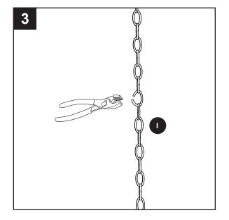
Unscrew the nut on open link (H), connect the chain (I) to the decorative rod (B), then close the open link (H). Weave the wires from the fixture (A) through the loops of the chain (I).
