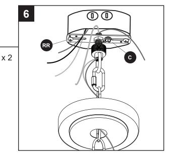
7. Loosen the ground screw on the mounting bracket (C) and wrap the bare wire from the fixture around the ground screw. Tighten the ground screw to hold the bare wire in place. **Note:** Ensure there is enough of the bare wire extending from the ground screw to connect to the ground wire from the outlet box using a wire connector.
