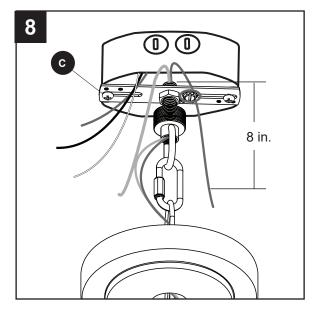
Separate the two fixture wires all the way to the mounting bracket (C). Strip 1/2 in. of insulation from the end of the wires. Twist the stripped ends of each strand of wire within the insulation with pliers (not included).
