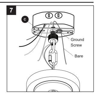
8. Depending on the length of chain (I) you use, you may need to cut the lead wires back to simplify the wiring. Take the lead wires and make sure that you have pulled them all the way through the top of the mounting bracket (C) and measure 8 in. of lead wire, and then cut the excess wire off with wire cutters (not included).
