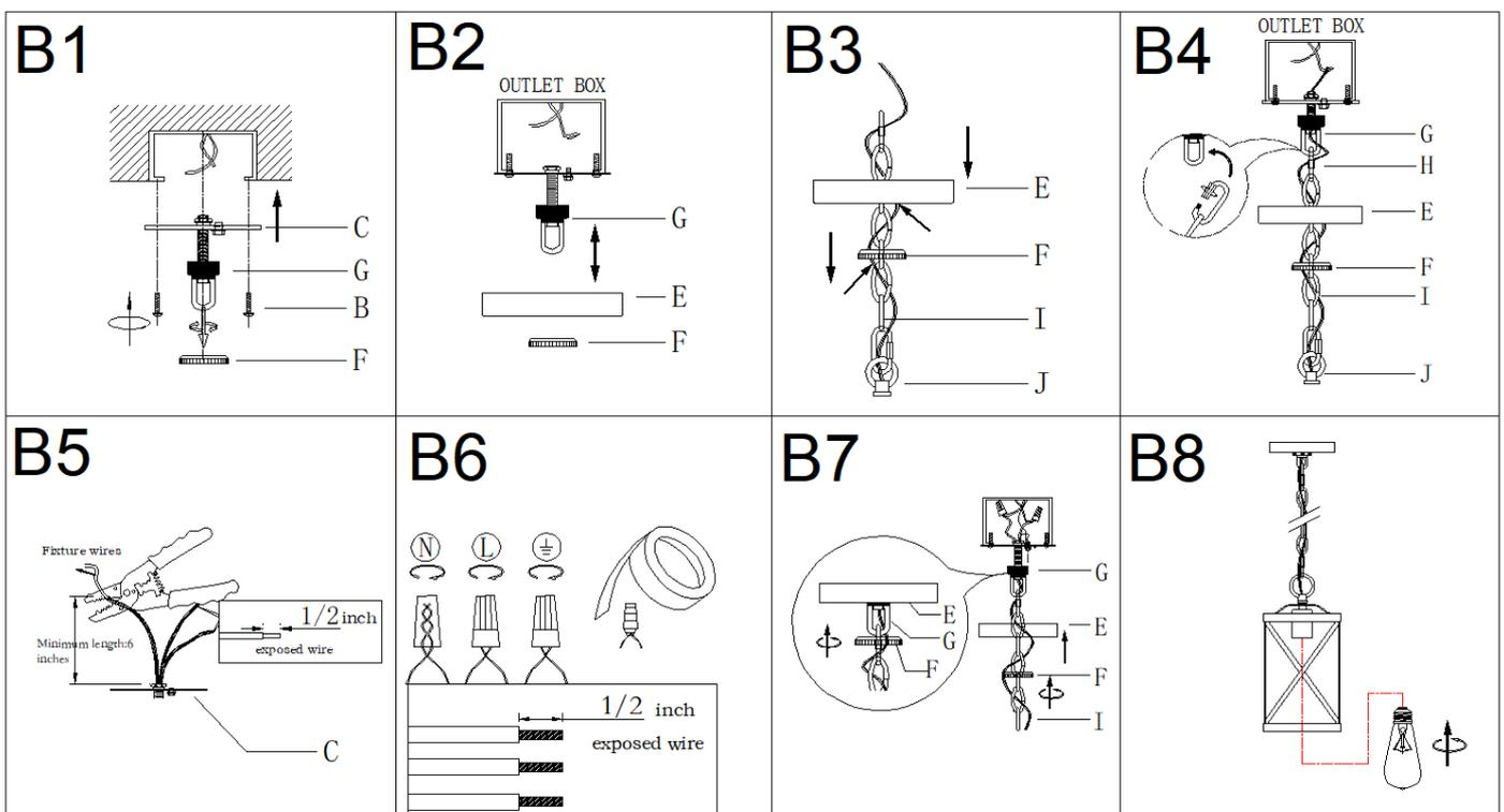
Step B1: Remove collar ring (F) from collar loop (G). Attach single bar (C) to the outlet box with mounting screws (B).
