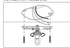
Detach the screw collar from chain holder. Mount the Crossbar kit together with the Chain holder using the Mounting Screws.
