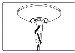
7. Put the Canopy back up against the ceiling and lock it in place using the Collar.
