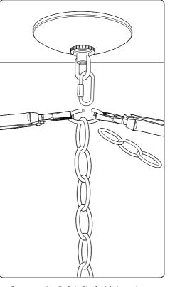
3. Connect the Quick Chain Link to the Chain Holder. Determine the height you want to hang the fixture down from the ceiling. Use a pair of pliers to twist to open the chain link end and remove the unwanted portion of Chain. Connect the wanted Chain to the Quick Chain Link. Twist to close both opened Chain Links.
