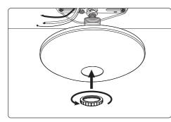
2. Attached the Canopy to the ceiling using the Screw collar.
