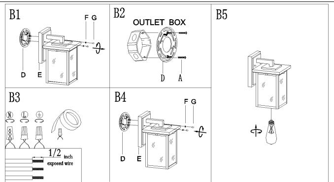
Step B1: Unscrew knob nuts (G) and remove plastic washers (F) from mounting plate (D), then set aside for the following steps.
