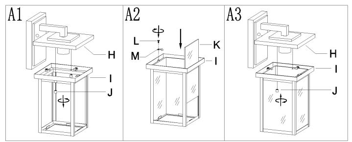
Step A1: Unscrew nut (J) and remove iron frame (I) from cover (H).
