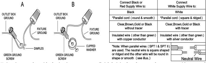
Twist wires together with plastic wire connector until tightly joined, and wrap each connector with approved electrical tape. Be sure that no wire strands are exposed and then carefully tuck all wires into the outlet box. Step B4: Align the holes in the back plate (E) with the pre-assembled mounting screws, then attach the back
