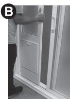
Step 2: Once the Pet Patio Door Panel is completely inserted into the top and bottom tracks and gently (C) slide the pet patio door panel to the side until it is secure in the side track channel. Note: if you sliding patio door lock catch (D) is interfering with the Pet Patio Door Panel, you can remove the lock catch or place the (2) Door Spacer Inserts (E) into the pet panel side channel, one approximately 18" from the top and one approximately 18" from the bottom.
