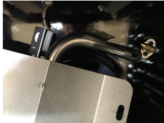
c. One screw on the front holding the broiler burner; d. Lose the four screws on flame tamer to get access to broiler orifice.
