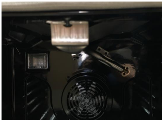
c. One screw on the front holding the broiler burner; d. Lose the four screws on flame tamer to get access to broiler orifice.
