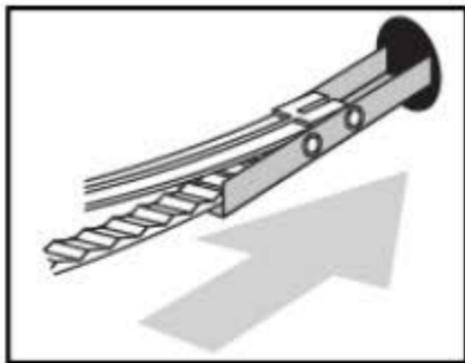
**1.** Identify and mark anchor location; drill a ½" diameter hole. Fold metal toggle against plastic strap and insert through the drilled hole.
