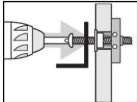
**5.** Place fixture mount over the flange, insert bolt\*, and tighten against fixture. Ensure bolt length is at least ½" longer than the combined thickness of your fixture and wall or ceiling.
