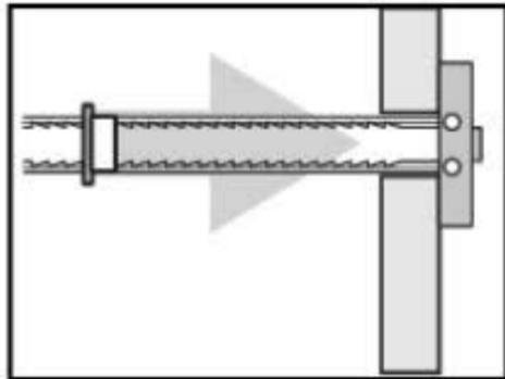
**2.** Pull end of straps away from wall or ceiling until toggle sits flush against the back of your wall or ceiling.
