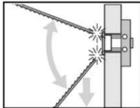
**4.** Gently separate straps and bend straps away from one another at the point where the strap meets the cap. Do not wiggle the straps or break in same direction. Broken straps can be discarded.
