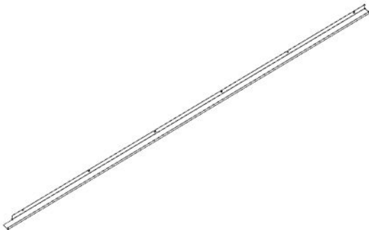
G02 GUTTER - A4M03481 (x1) 1 9/16"x1 15/16"x111 13/16" (40x50x2839)
