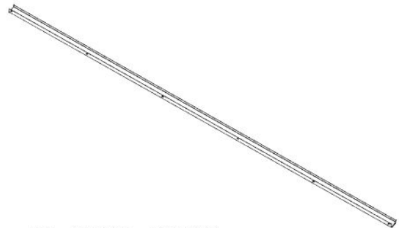
G03 GUTTER - A4M04120 (x1) 1 9/16"x1 15/16"x111 11/16" (40x50x2837)
