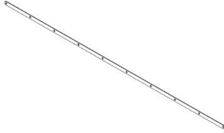
F02 LOUVER TIE STRAP - A4M04121 (x2) 1/8"x13/16"x61 3/8" (3x20x1559)
