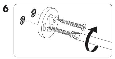
Install the mounting plate with the provided screws.
