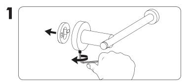
Remove mounting plate from back of toilet paper holder. **a.** Use the provided allen wrench to loosen set screw on bottom of the toilet paper holder to remove the mounting plate. Level and mark position of the toilet paper holder on the wall. **a.** If mounting into ceramic or tile, place masking tape on the mounting areas before marking the location to prevent the drill from slipping and damaging the tile.
