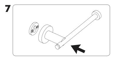
Place the toilet paper holder over the mounting plate with the set screw on the bottom.
