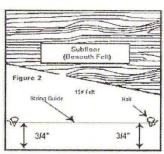
**Note:** This dimension should be 4" when installing 3 ¼" wide flooring. When a room is greater than 20 ft. in width, the direction of the installation should start near the center of the room and work out towards the walls Placing a loose spline where the two grooves come together.
