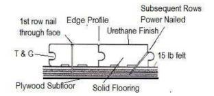
NOTE: DO NOT USE A RUBBER MALLET TO INSTALL FLOORING. STRIKING THE SURFACE WITH A RUBBER MALLET MAY "BURN" THE FINISH CAUSING IRREPARABLE DAMAGE
