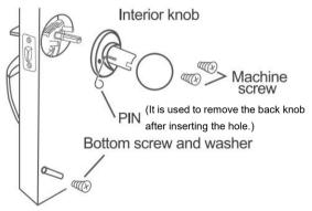
After the front handle is in position, install the interior knoband tighten screws. Insert screw through washer and into bottom hole tighten firmly.
