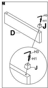
Attach wood legs "J" with footboard "D". Using Allen key (H3) to lock with bolts "H1".
