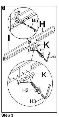
Attach wood bar "K" to the 2 rails "H" & "I". Using Allen key (H3) to lock with bolts "H2". Lock the both side rails ( H & I) (front & rear of rail) tight and alignment with
