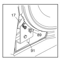
Reattach the parts that you removed. Then, plug in the power adapter.
