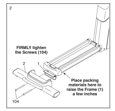
3. With the help of a second person, place some of the packing materials (not shown) under the front of the Frame (1).
