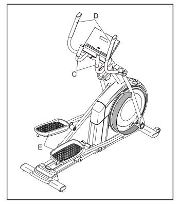
To dismount the elliptical, wait until the pedals (E) come to a complete stop. Note: The elliptical does not have a free wheel; the pedals will continue to move until the flywheel stops. When the pedals are stationary, step off the higher pedal first. Then, step off the lower pedal.
