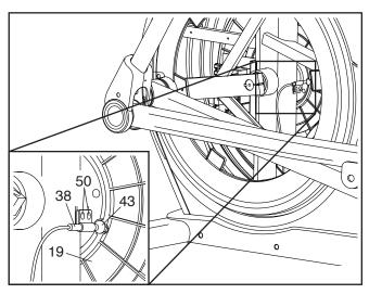
Then, plug in the adapter and rock the Pulley (19) forward and backward just enough that the Magnet (43) passes the Reed Switch (38) repeatedly. Repeat these actions until the console displays correct feedback.
