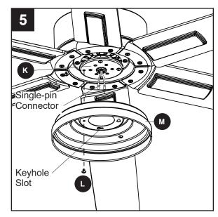
6. Remove one and loosen the other two light pan screws (N) from the underside of the light pan (M). Connect the single-pin connector from the fitter plate (K) to the single-pin connector from the light kit (O) --blue to black and white to white. Align the keyhole slots in the light kit (O) with the loosened screws in the light pan (M). Turn light kit (O) clockwise and replace the previously removed light pan screw (N). Tighten all screws.
