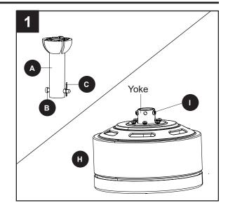
2. Insert the downrod (A) -- or a longer downrod (not included), if required -- through the canopy (E) and yoke cover (G). Feed the wires from the fan through the downrod (A).
