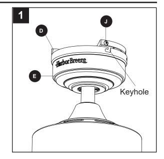
2. Secure the canopy (E) with the mounting bracket screws (J) previously removed (Step 4, page 8). Tighten all mounting bracket screws (J) securely.
