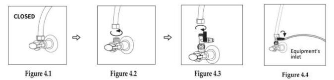
**NOTE:** Never install a water supply connector on a hot water line.
