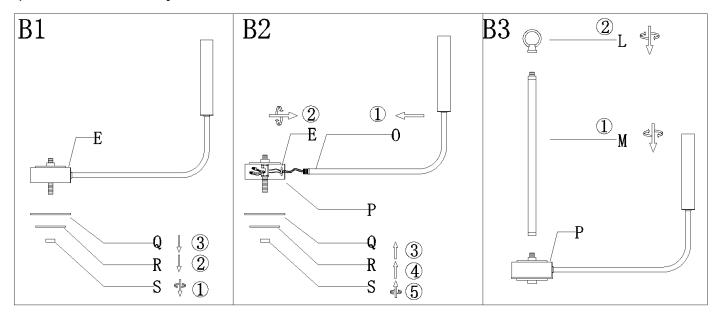
Sept B1:Unscrew the finial (S) from fixture body (P)then remove the bottom trim (R)and lid (Q) from fixture body (E)
