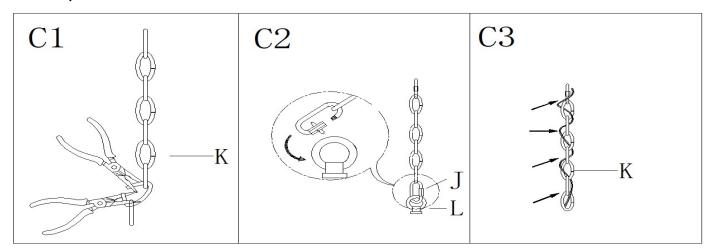
Step C1: By measuring, determine the correct number of links needed for proper hanging height. Using the chain pliers, disconnect and discard the remaining chain.
