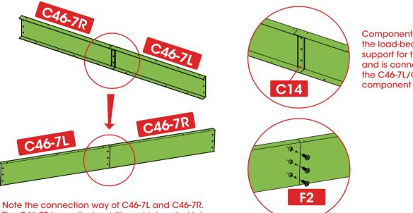
Component C14 is the load-bearing support for the roof and is connected to the C46-7L/C46-7R component joint.
