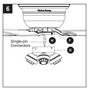
7. Secure the light kit (G) to the fitter plate (F) by reinstalling the fitter plate screws (N).
