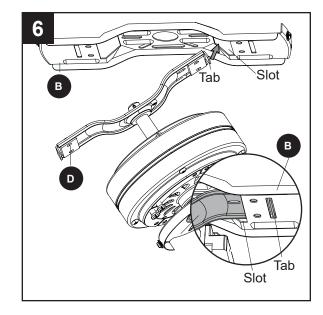
7. Re-install the previously removed lower bracket screws (M) to secure the lower mounting bracket (D) and the upper mounting bracket (B).
