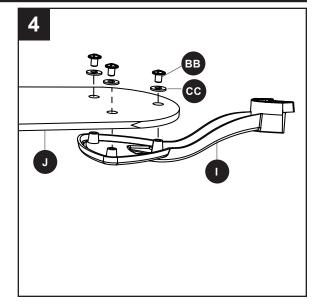
Install the blade arm (I) to the underside of the motor (E) with motor screws (L) previously removed (Step 3, page 10). Tighten with Phillips screwdriver.
