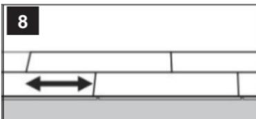
9. Second plank second row. Place the panel gently and close to the short end of the previous panel and fold it down in a single action movement.
