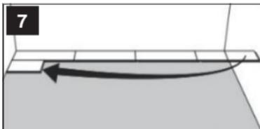
8. Staggered joint distance i.e. minimum distance between short ends of planks in parallel rows shall NOT be less than the given width of the plank.
