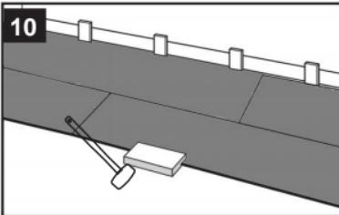
11. After 2-3 row. Adjust the distance to the front wall by placing spacers. Ensuring a 0.1574-0.1967" expansion gap.
