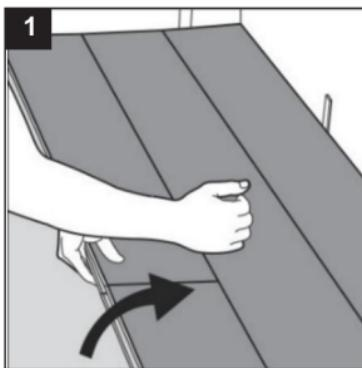
2. Disassemble the panels by lifting up under the short end.
