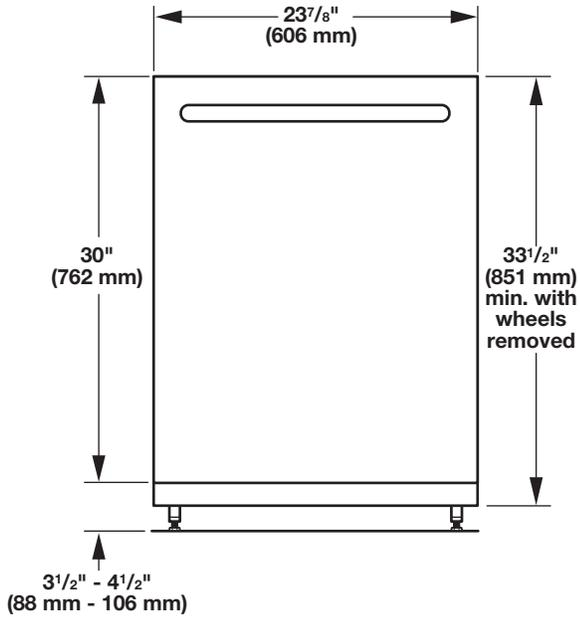
For 4" (100 mm) toe kick, height of cabinet opening is 34<sup>1</sup>/<sub>2</sub>" (863 mm).
