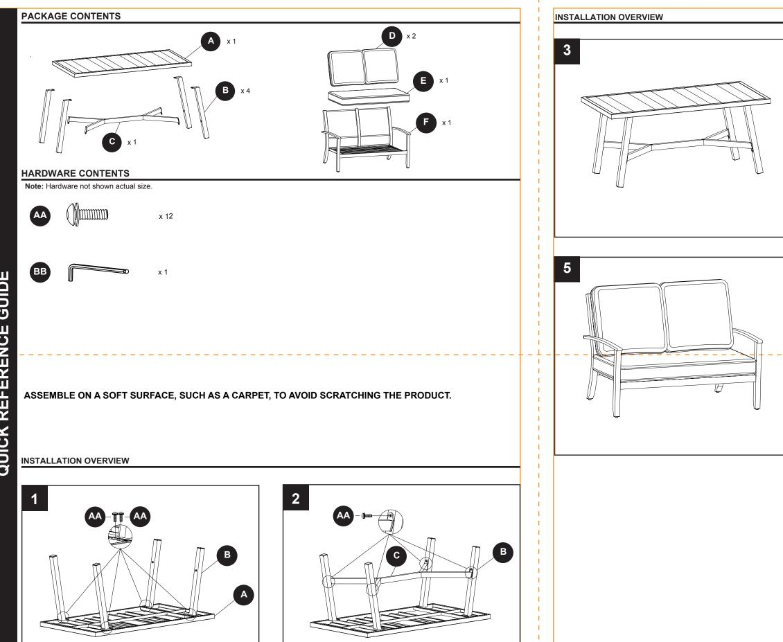
Hand tighten AA. Do not tighten until all bolts have been installed.
