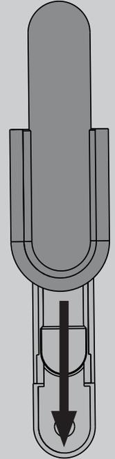
Slide the cradle onto the mounted bracket.
