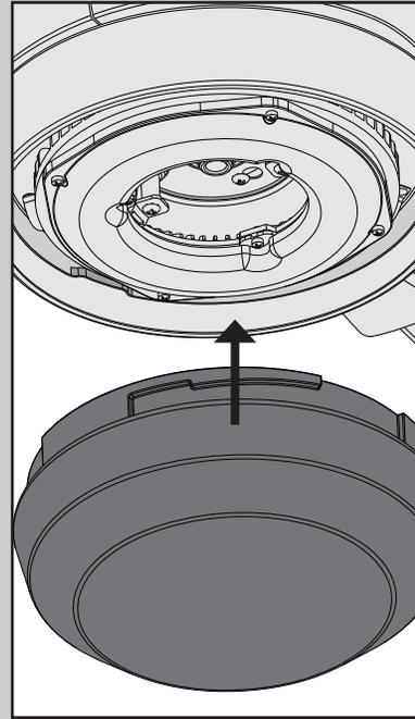
Lift the globe and align the notches in the globe with the tabs in the light kit. Attach the globe by lifting and twisting clockwise until it rests firmly in place.
