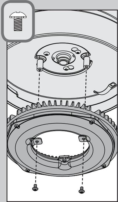
Raise the LED assembly to the posts in the housing. Attach the LED assembly using the LED assembly screws found in the hardware bag.
