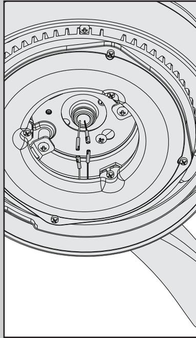
Connect the white wire from the fan to the white wire from the light kit. Then, connect the blue wire from the fan to the black wire from the light kit.
