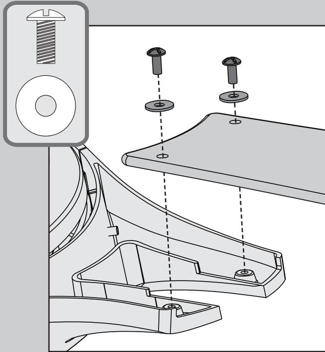
Put the blade washers found in the ■ hardware bag onto the blade screws found in the ▲ hardware bag. Then install the blade screws to secure each blade to a blade iron.
