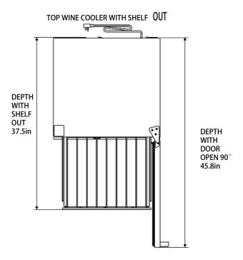
Keep enough clearance between the appliance and its surroundings to ensure the function of the appliance.
