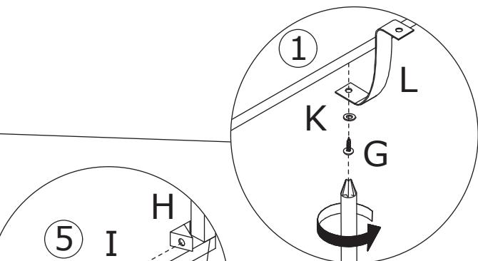
Insert buckle(H) into back slots and fix with screw(I) as shown. Fix strip(L) to board 1 through washer(K) with screw(G) as shown.
