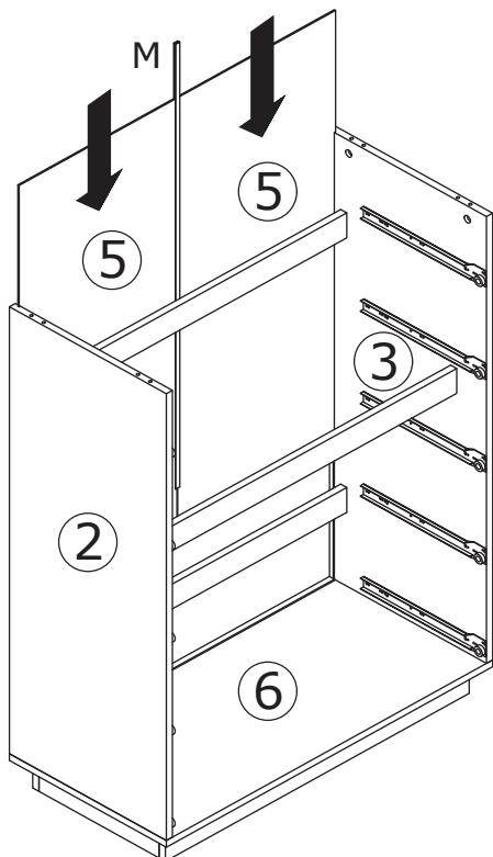
Connect each board 5 to plank(M) at first. Insert back boards along available grooves as shown.
