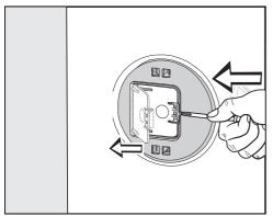
Press against the catch with a thin object (a narrow screwdriver, for example).
