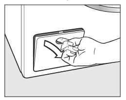
Open the drain pump flap.
