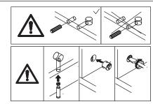
Insert wooden dowel B into board 7 and board 8, and connect board 13 with board 7 and board 8.
