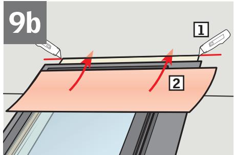
**ENGLISH:** To allow for proper drainage, interweave VELUX adhesive skylight underlayment as shown in **9a** for new construction applications. For retrofit applications, interweave VELUX adhesive skylight underlayment as shown in **9b**.
