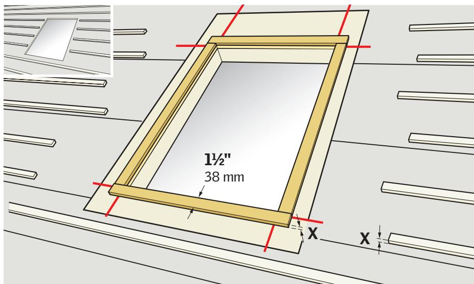
**ENGLISH:** Roof with battens: Place 1 1/2" (38 mm) wide battens around rough opening. Batten thickness around rough opening should be equal to thickness of battens used for roofing material.
