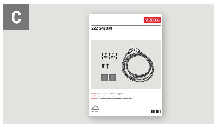
**ENGLISH:** For steep roof pitch above 45° (12:12) use wire extension kit ZZZ 241DM to relocate the solar panel and rain sensor as shown in the enclosed instructions for ZZZ 241DM.
