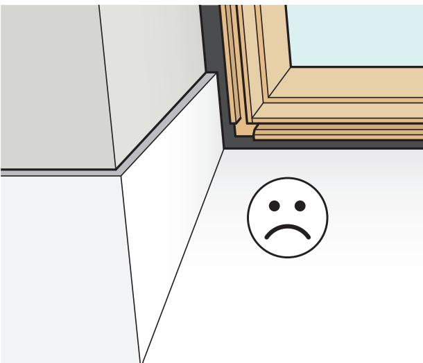
**ENGLISH:** Drywall not installed properly into the lining groove.
