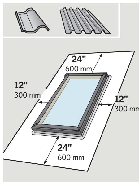
**ENGLISH:** For skylights provided with an insect screen, a flared light shaft is required to remove the insect screen. See details.
