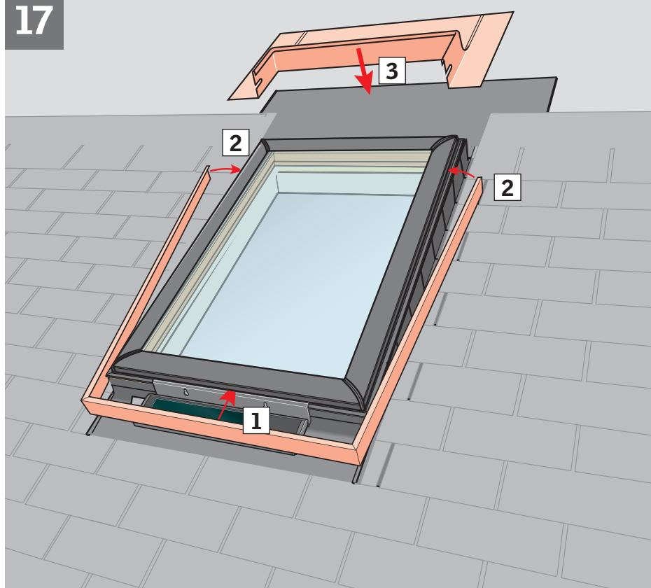
**ENGLISH:** Reinstall cladding (1), (2) and continue installation of flashing (3).
