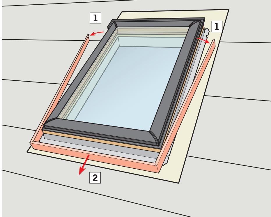
**ENGLISH:** Center skylight over properly cut and framed rough opening using alignment notches as shown (a). Anchor skylight with 1 1/4" (30 mm) nails provided with the skylight, one nail per pre-punched hole in mounting flange. The carbon steel nails are zinc-coated (double hot-dipped).
