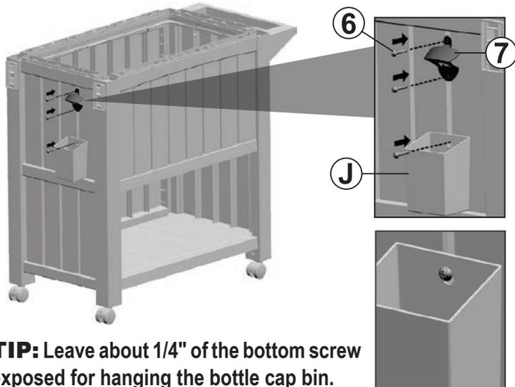
**TIP:** Leave about 1/4" of the bottom screw exposed for hanging the bottle cap bin.
