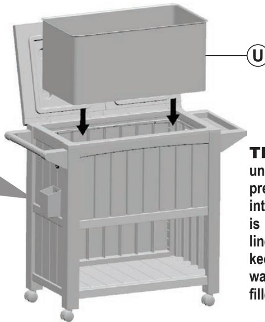
**TIP:** Locate the lip just under the cooler rail and press the top of the cooler into the indentation; this is not a firm hold of the liner, it is intended to keep the rim out of the way while the cooler is filled with ice.
