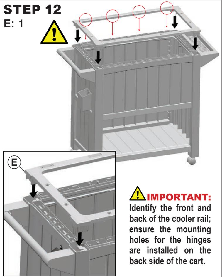
**! IMPORTANT:** Identify the front and back of the cooler rail; ensure the mounting holes for the hinges are installed on the back side of the cart.
