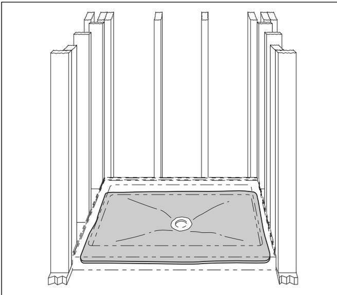
2. Place the shower floor into the rough opening and firmly press it into the mortar/thinset. The exposed front bottom edge(s) of the shower floor should contact the subfloor.
