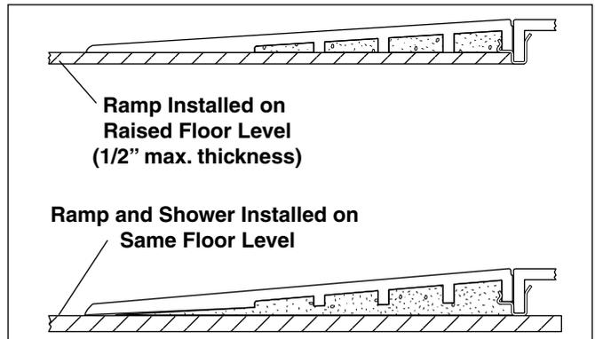
7. Firmly press the barrier-free shower floor ramp into the mortar/thinset. The back (tall) edge of the shower ramp must engage all eight of the stainless steel clips to prevent the shower ramp from moving. The front (thin) edge of the shower floor ramp must completely contact the floor surface.
