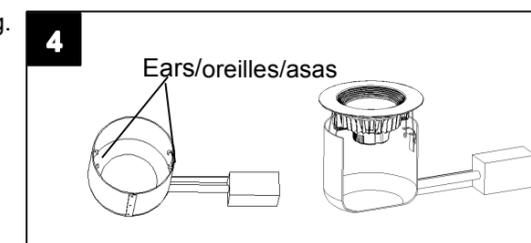
5. Carefully route wires into fixture. Push retrofit into recessed housing until the trim is flush with the ceiling surface.
