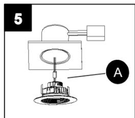
6. Carefully route wires into fixture. Push retrofit into recessed housing until the trim is flush with the ceiling surface.
