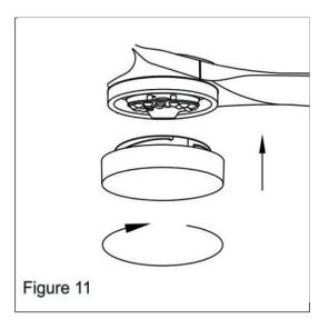
10. Tighten the canopy with two screws.
