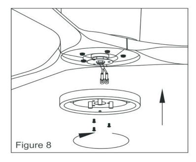
3) Connect the LED lighfs wires to the fan motor's wires. Tighten the LED with screws removed in step 1).
