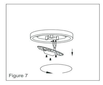
2) Align the screw holes of the lamp holder with that of the motor, and attach both parts by the screws provided.
