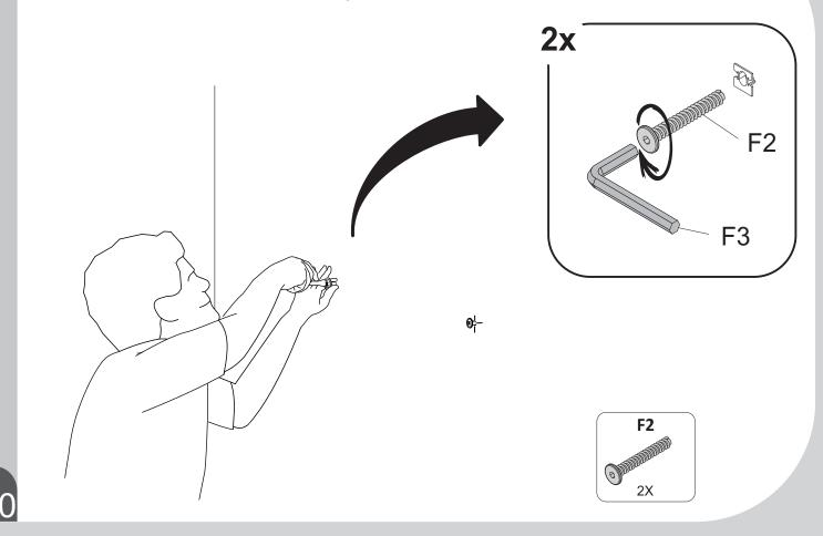
1- Approach the cabinet by fitting the F2 screw.
