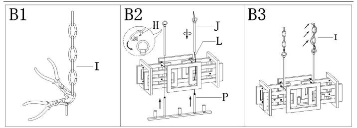
Step B1: By measuring, determine the correct number of links needed for proper hanging height. Using the chain pliers, disconnect and discard the unwanted part.
