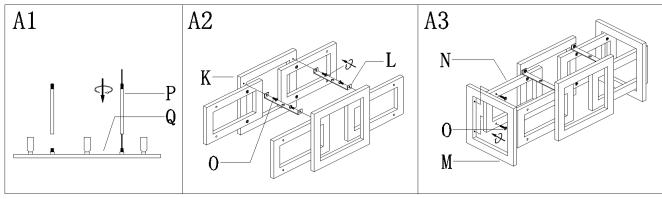
Step A1: Pass the fixture wires through stem (P) and then screw stems (P) onto fixture body (Q).
