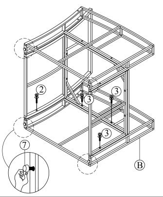
Connect Part from STEP 4 & Left Frame (B) with Bolt (1) & Washer (6)
