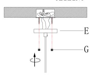
9 » Install the bulb (Not included) (Please do not exceed the maximum wattage recommended on the socket.)
