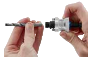
STEP 2 Unlock Pilot Bit
