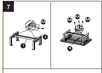
Once all connections are made, tighten AA with CC.
