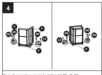
Once all connections are made, tighten AA,BB with CC.
