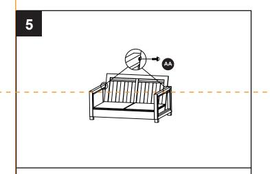
Once all connections are made, tighten AA with CC.
