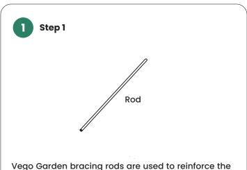
Vego Garden bracing rods are used to reinforce the strength of long raised beds. For the 11 inch 9 in 1, only the 2ft wide configurations need a rod.
