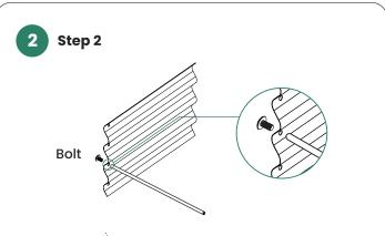
Install the bracing rod between two parallel bolt holes. Attach bolt, panel, washer & rod loosely, making sure that the rod is connected in the **third** bolt hole from the top. Then tighten it up with the screwdriver for reinforcement of raised bed.
