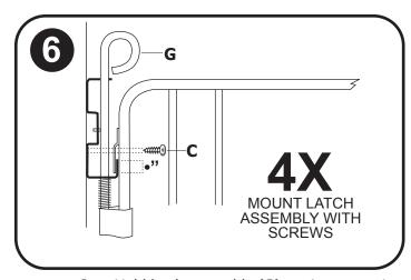
Hold latch assembly ( $\mathbf{G}$ ) against opposite wall and extend gate until at least  $\frac{1}{2}$ " of safety bracket will interlock with flange of latch. Mark position of latch assembly screw holes with pencil. Swing gate out of way and mount latch assembly to wall. Check closure of gate and tighten set screws from STEP 5 to secure gate width.
