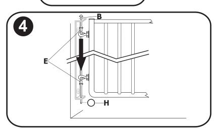
Hang gate by inserting hinge rod  $(\mathbf{B})$ , through top of mounted hinge bracket  $(\mathbf{A})$ , through upper plastic shoulder washer  $(\mathbf{E})$ , through both eye bolts, through lower plastic shoulder washer (E), and finally through bottom of hinge bracket. To secure hinge rod, insert key ring (H) through hole in end of hinge rod.
