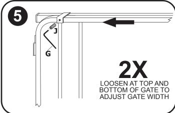
Set gate to width by holding latch assembly against 5. mounting wall (see beginning of STEP 6). Use Allen wrench(F) to insert set screws (J) and tighten top and bottom of gate.
