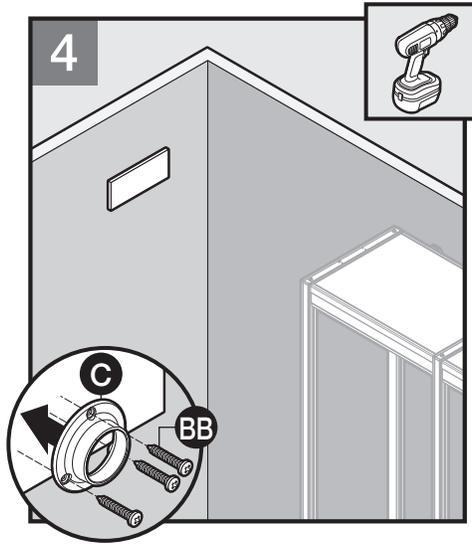
Attach the rod socket (C) to the installed cleat with the included screws (BB).
