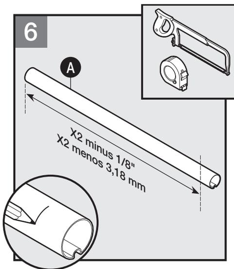
Mark measurement X2 (from previous step) minus 1/8" (for socket width) on the clothes rod (A). Using a hacksaw, cut the clothes rod (A).
