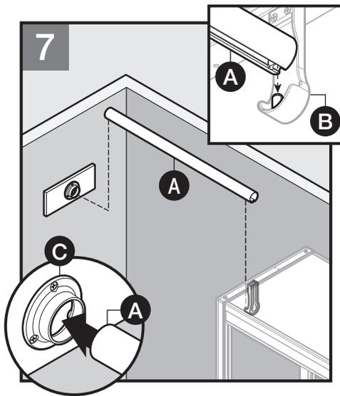
Insert one end of clothes rod (A) into installed pole socket (C). Slide the other end of clothes rod (A) straight down onto rod bracket (B), aligning rod holes with bracket pegs. It should snap firmly in place.
