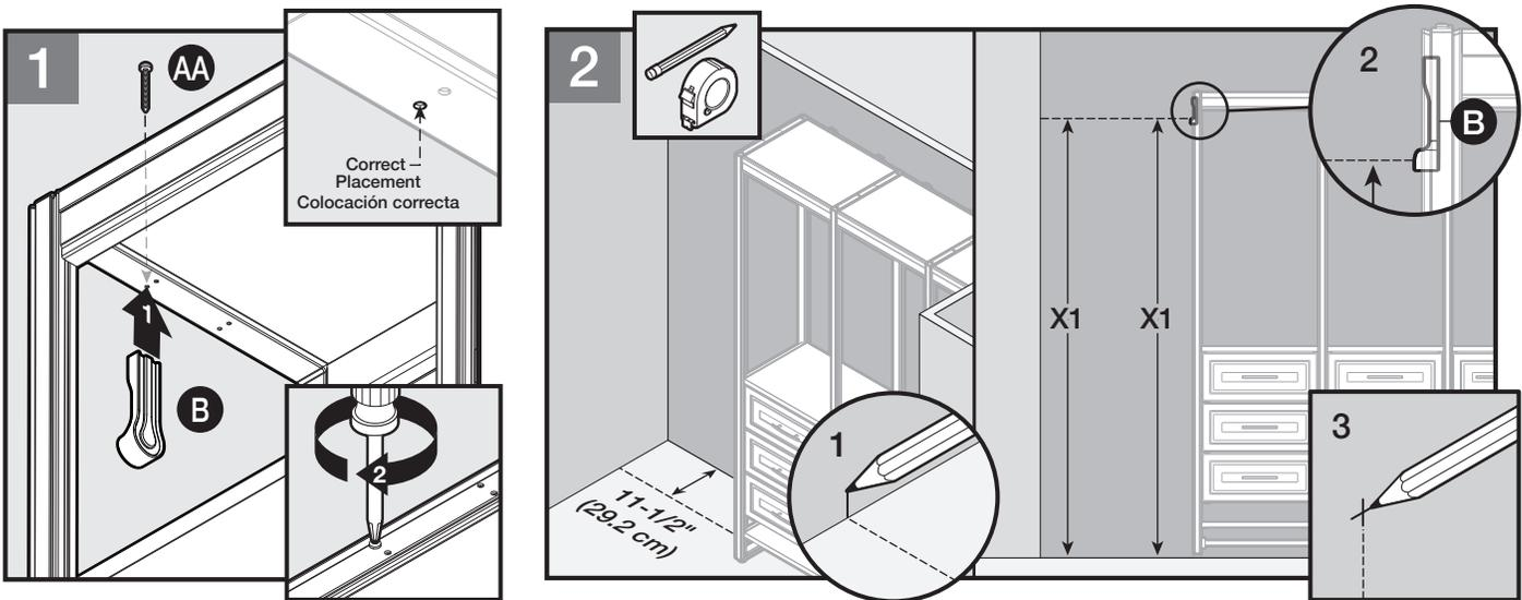
1 Install the rod bracket (B) by inserting screw (AA) through the top of the frame using the front hole closest to the middle of the tower. Tighten to secure.
