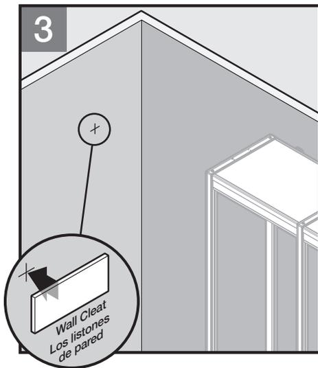
To insure proper installation, attach a wall cleat (not included) to closet side wall with screws and drywall anchors.
