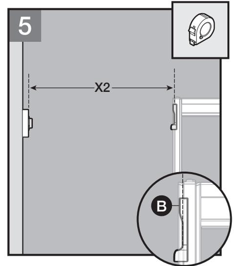
Measure the distance (X2) from the surface of the cleat to the inner edge of the rod bracket (B).
