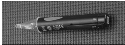
Use a non-contact circuit tester to check for electrical power.
