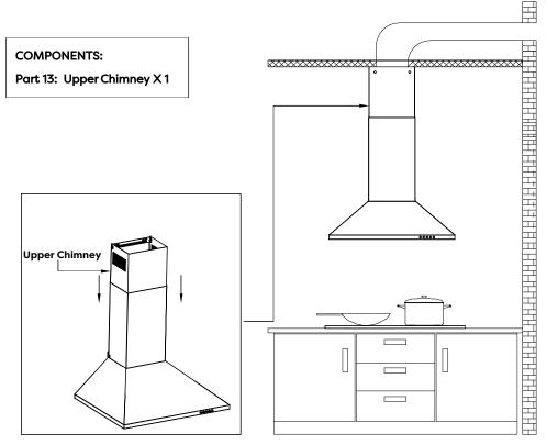
17) Use two 0.16"\*0.32" Screws to assemble the Upper Chimney on the Upper Chimney Bracket.
