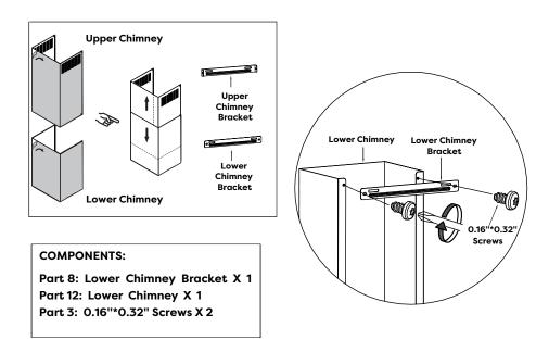
13) Insert the Lower Chimney into the hood and fix it to the corresponding positioning hole with two 0.16"\*0.32" Screws. (Note: That the power cord needs to go through the chimney and connect the power).
