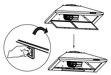
2. Place the carbon filter into the unit and turn it in the clockwise direction to lock it in place.
