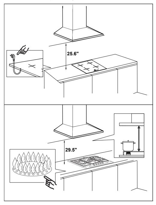
3) First use a pencil to mark the installation position on the wall, then use a Measuring Tape to measure the height from the stove surface to the hood (the center point of aluminum grease filter) and use a Spirit Level Ruler to maintain the level, then use a pencil to draw a horizontal line along the level.
