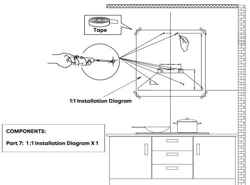
5) Determine the maximum chimney installation height according to the actual scenario and mark the chimney installation locations along the center line of the Installation Diagram.
