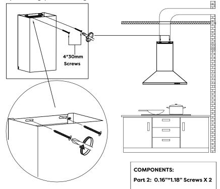
15) Use two 0.16"\*1.18" Screws to lock the Upper Chimney Bracket to the corresponding positioning holes on the wall.
