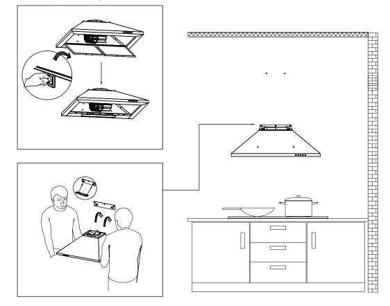
9) Use a Spirit Level Ruler to measure whether the hood is in a horizontal level, and use two 0.16"\*1.18" Screws to lock into the safety hole position of the hood (not mandatory, according to user's wishes to choose whether to lock).
