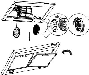
3. If the carbon filter needs to be replaced, please turn it in the anticlockwise direction.
