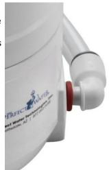
NOTE: to remove the elbow fitting stem from the base, depress the red collet ring fully against the base, while simultaneously, gently pull out the elbow. Very little force is required, but some wiggling and patience may be involved. Please do not use tools or brute force. **Please call for support 877-693-7873.**
